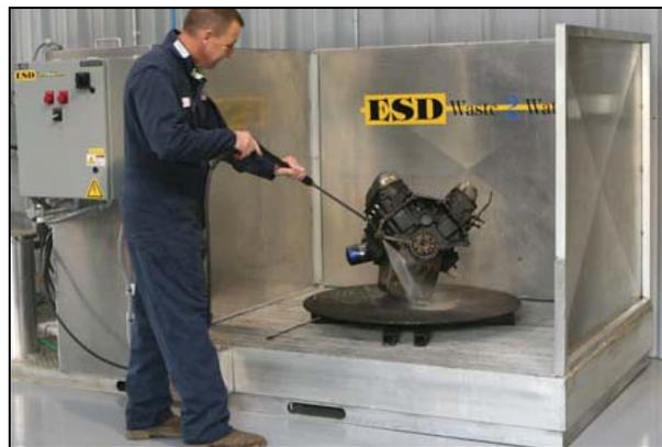
**Figure D3-1 Self-Contained Closed Loop Parts Washing System**
