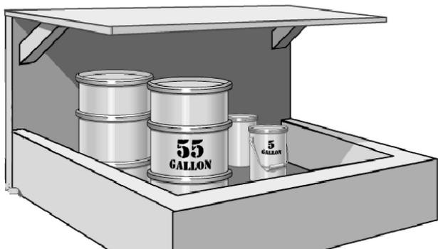
**Figure A2-1 Example of Outdoor Storage with Roof and Secondary Containment**
