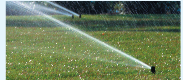
Properly functioning rotor sprinkler head
