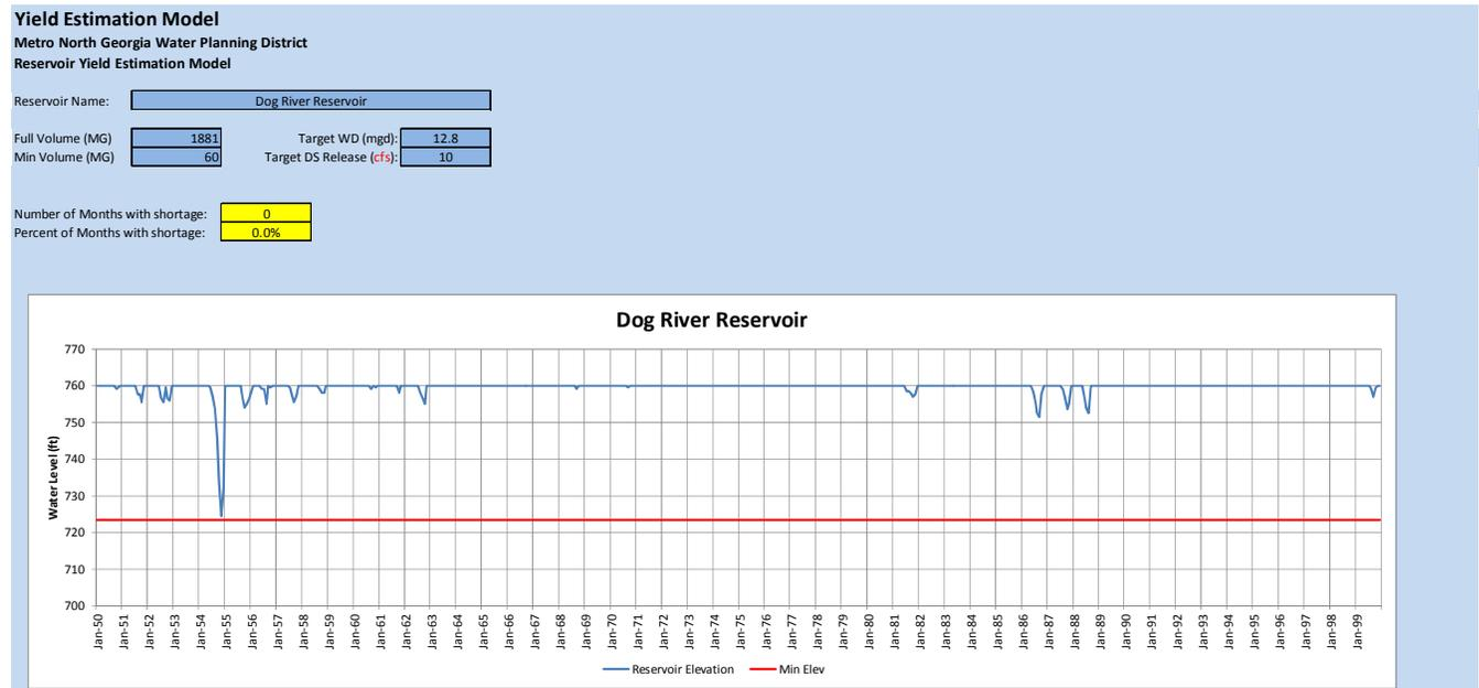
Figure 3.2.8 Example Reservoir Model Output (Sample results only)
